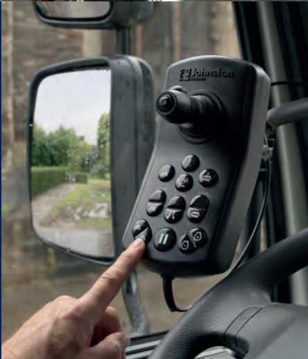
TOP Pendant control for safely raising the hopper
